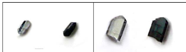
Figure 3. Photographs of 2a (left) and 3a (right) before and after UV irradiation at 365 nm.
